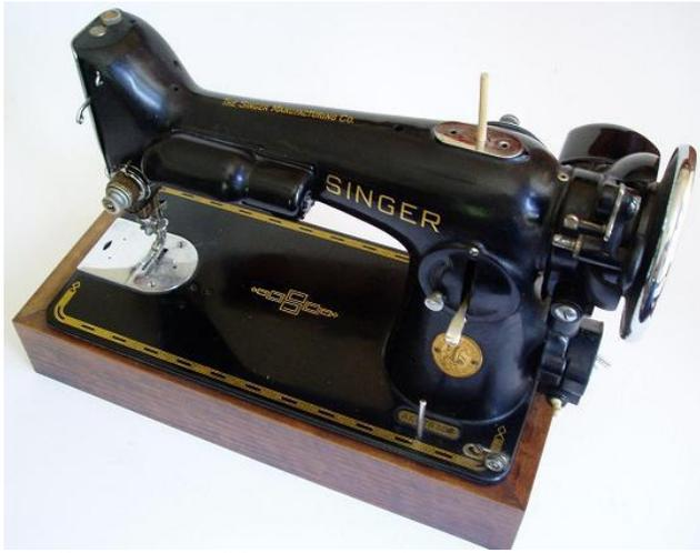
The Singer Model 201 is perhaps the finest sewing machine ever built. It is solid, gear-driven, and heavy, which means it sews very smoothly.
