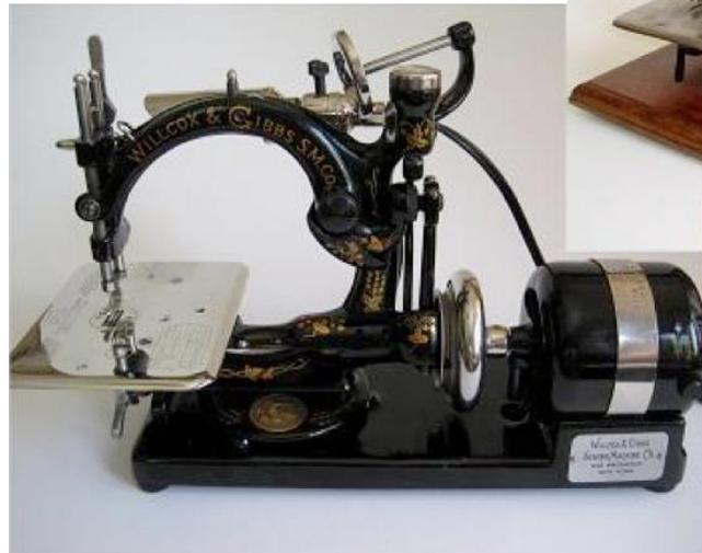
Willcox and Gibbs was another early sewing machine manufacturer. Their machines changed very little over the years. This composite shows the three common ways in which sewing machines were powered: treadle, hand crank, and electricity. Willcox and Gibbs was the undisputed leader in quality chain stitch machines; therefore a number of companies made copies of the machine when the patents expired, and even Singer was forced to come out with a competing machine.
