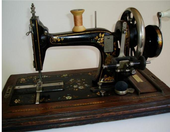
German Gritzner from about 1900 was called a "High Arm" machine because the arm was raised a bit higher than on the Singer Model 12. The rest of the sewing mechanism was copied from the Model 12, which first came out in the mid 1860s. Much of the decoration on the bed of this machine is not paint but is inlaid Mother of Pearl.
