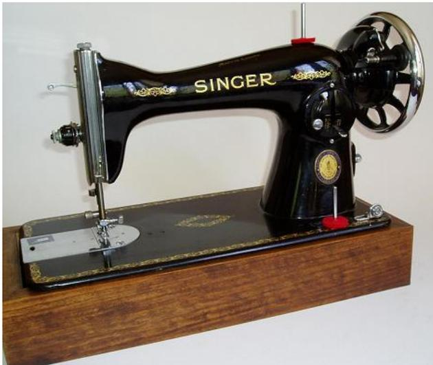
This is a Singer Model 15 from 1951. The badge on the machine identifies it as a centennial machine marking the 100th anniversary of the Singer Company. The Model 15 can be identified from other Singer models because the tension control sticks out to the left as you sit at the machine ready to sew. The Japanese HA-1 machines are nearly an exact copy of this machine.
