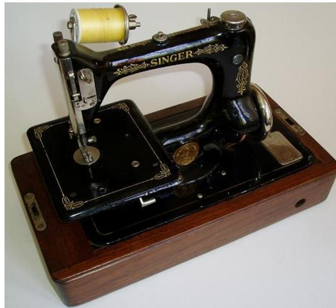
The success of the Willcox and Gibbs machine obliged Singer to come out with a competing machine once the Willcox and Gibbs patents had expired. The mechanics were largely based on the Willcox and Gibbs machine. This is an electric Singer Model 24 from the 1920s. The motor and speed controller were hidden under the plate, and the hole on the right side of the case was for a knee lever to operate the controller.
