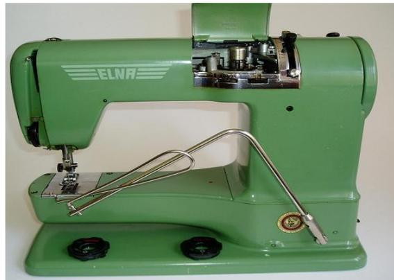
The Elna Supermatic from Switzerland was introduced in the early 1950s. It could not only do straight and zig-zag stitches but a large number of decorative stitches by the insertion of various special cams.
