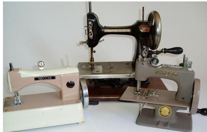
A number of sewing machines were built for children. Nearly all toy machines were hand crank. The Little Worker (in back) sewed with a lock stitch and could actually be used as a small portable machine. The Singer design (right) was actually based on the Willcox and Gibbs machine and sewed with a twisted chain stitch. It could also be used to actually sew clothes. The Necchi (left) was used to promote Necchi's larger machines and is only a toy.
