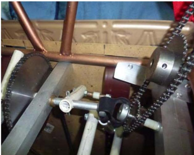
Drive shaft connected to secondary shaft with universal joint coupler
