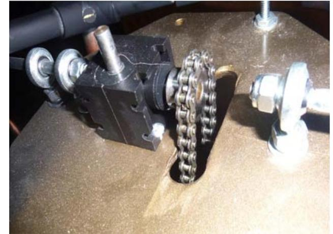
Gear box at top, and propeller shaft.
