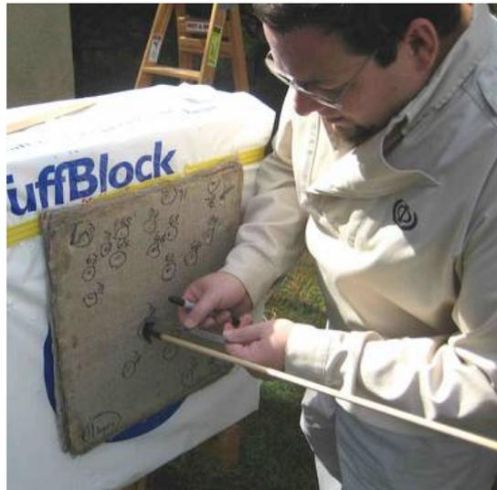
Patch of laminated material hung on dense foam block simulating a human torso. (left) Measuring penetration. (right)
