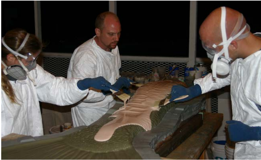
Pouring Bondo before adding fiberglass onto clay sculpting.
