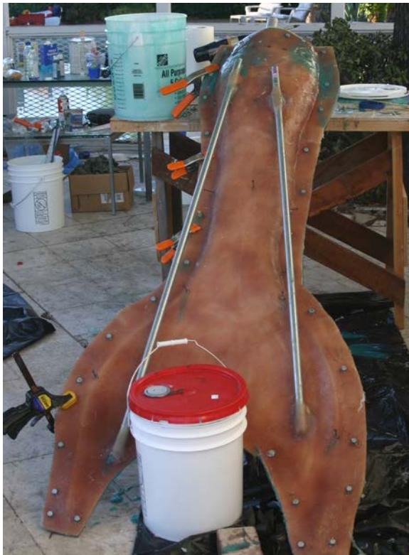
Above: Pouring phthalo green tinted silicone. Below: Halves of mold bolted together, during silicone pour.
