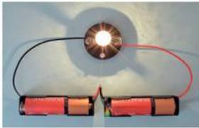
Figure 2-7: The most common way to connect batteries is in series. This increases the voltage. We have two 1.5V batteries, so our lamp is receiving 3V of power, which makes it shine twice as brightly and risks burning it out. Battery holders connect the batteries in series; a four battery holder will give you 6V, an eight battery holder will give you 12V, etc.
