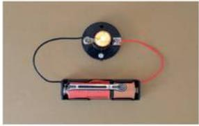
Figure 2-4: A single AA battery provides 1.5V. When we hook up a 1.5V lamp to it, it shines happily at full brightness.
