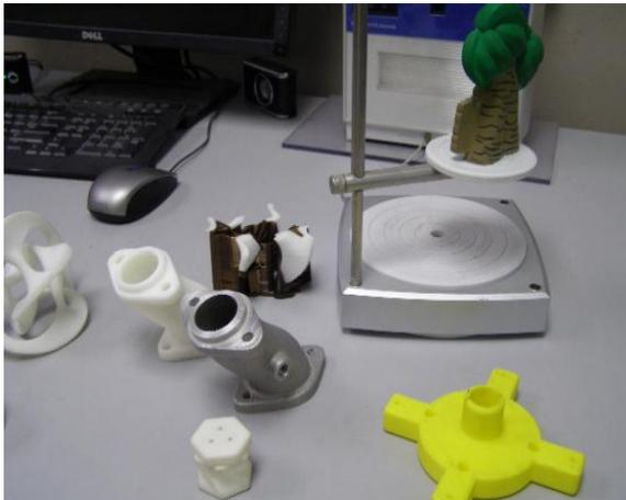
These files can be used in a variety of millers available elsewhere in the building, or in the 3D printer also housed in this room. Scans can be used at natural size or scaled.
