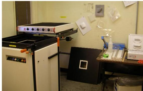
No, I don't have an inner Stormtrooper that I need to let out, but there are so many costumes where I duplicate vacuum formed objects by hand, that I am eager to finally get a whack at it myself. This machine is industrial grade, will heat the plastic automatically, and has multiple windows that can be inserted to enable almost any size plastic sheet you want to use
