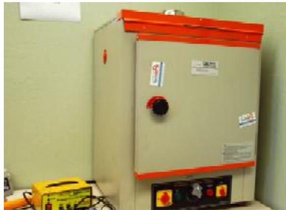
This room also has the equipment for powder coating, a process in which a fine plastic powder is sprayed onto metal objects, adhering by an electrostatic charge, then baked on for a firmer hold than spray paint.
