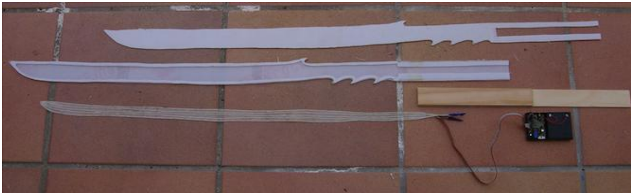
Sword made of clear acrylic plastic with embedded blue EL wire array and electronics.
