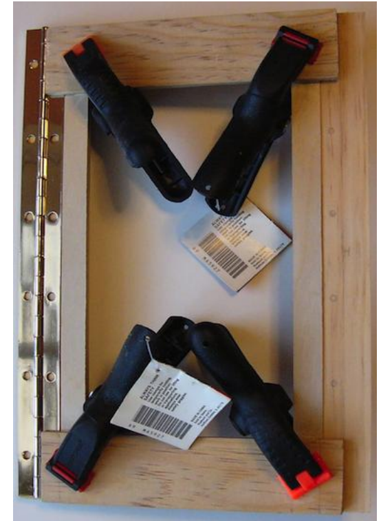
Glue the box frame together, leaving room for hinges on both edges (above). Attach the wings to molding pieces attached to the hinges (below).
