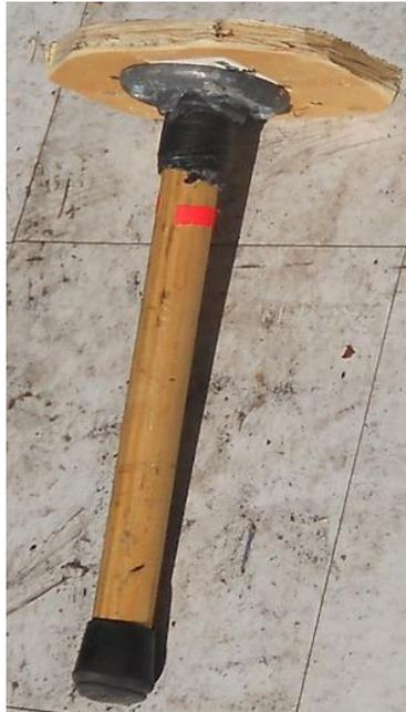
Peg assembly: closet dowel, table flange, plywood, and rubber tip.
